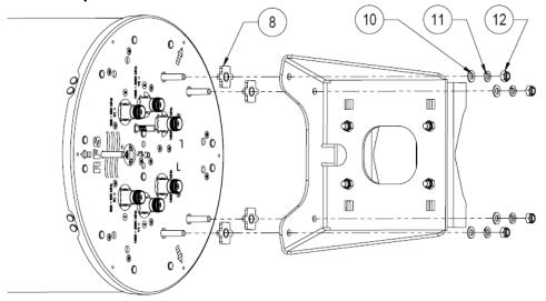
3. Connect item3 to above sub-assembly by M12 screw, washer and nut (No need to tight).
